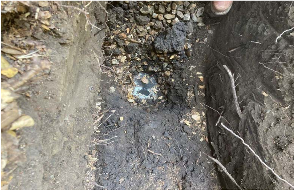
Photo 3: OWS 1 Wastewater Flowing Out after the Distribution Lateral Pipe was Perforated to Introduce the Tracer
